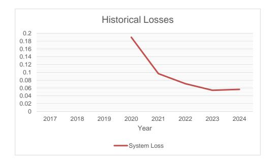
The system loss remained low in 2024 with an average system loss of 5.65%. The overall system loss of MORE Power's was maintained at low levels due to continued effort to upgrade the distribution system and its unwavering campaign against pilferage to further reduce the overall system loss to within the cap.
