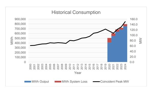
MWh Output in 2024 is 749,692 MWh, while the System Loss is 44,876 MWh equivalent to 5.65%. This is an improvement from the 679,452 MWh Output in 2023 and a system loss of 44,876 MWh equivalent to 5.65%.
