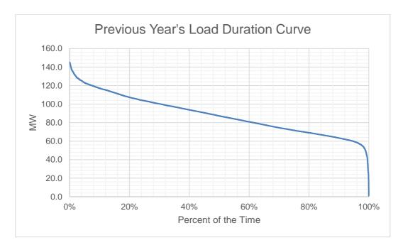
The Load Duration Curve of 2024 is shown above. The minimum load is 4.37 MW. This occurred during the Panay-wide power outage on Jan 2, 2024, caused by grid disturbance and multiple outages of power plants.
