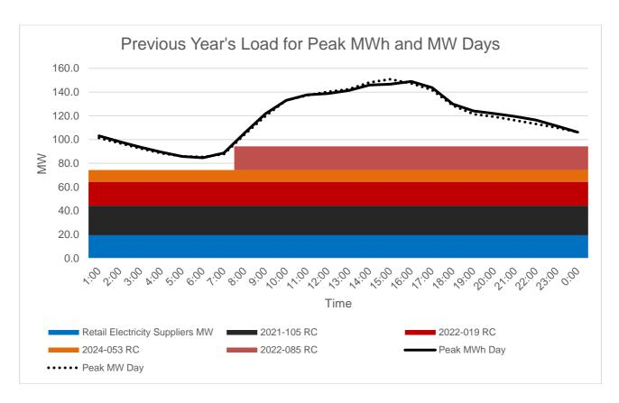
In 2024, the peak demand reached 151 MW on May 22, based on the NGCP meter at 5-minute interval. The highest energy consumption in a single day (peak MWh day) occurred on May 21. As shown in the Load Curves, the available supply was lower than the peak demand. Baseload requirements were supplied by Sem-Calaca, KEPCO SPC, and PEDC, while EDC provided mid-merit capacity. The remaining power supply was sourced from WESM.
